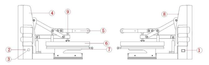
① Digital Controller④ Power Switch⑦ Base Plate
