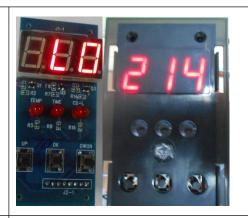
When rising to the set temperature, close down the heat platen and time controller starts to countdown.. Tips: it will show LO when temperature is below 100°C.
