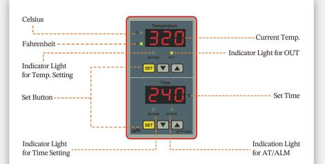
(The maximum temperature can be set to 491°F, and 255°C. The suggested curing tempera-
